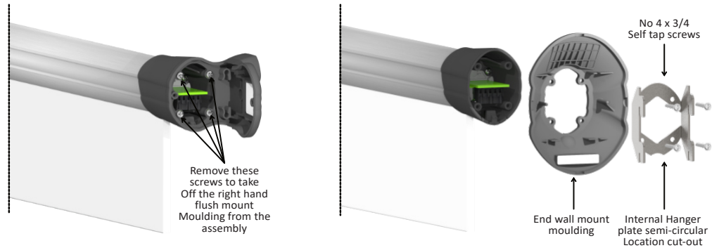
Fig 5-3: Removing the Left Hand Assembly
