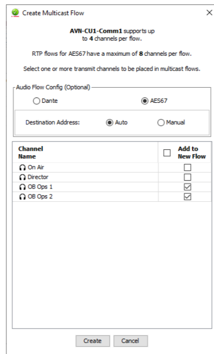
Fig 7-14: Creating a multicast flow In the example, the channels OB Ops 1 and OB Ops 2 are added to the AES67 multicast flow. When the required channels have been selected, press the Create button.
