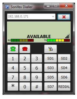
The dialler has a numeric keypad, speed-dials, last number re-dial, Rx and Tx metering, status indicator.
