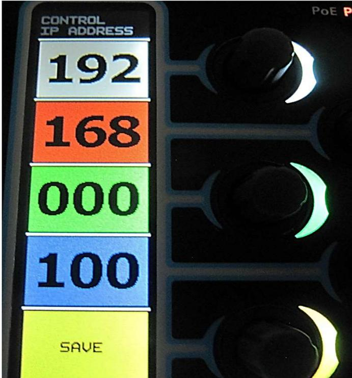
24. Using the rotary buttons next to each of the locations adjust the IP address to suit your network.
