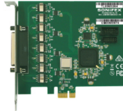
The PC-DIG4 Digtorc 4, 4 Stereo AES-3 I/O PCIe Sound Card
