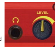
Fig 4-9: RB-DMX4 Headphone Output & Level Control
