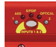
Fig 4-5: RB-DMX4 INPUT 1 & 2 Select Button
