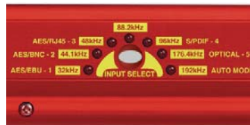
Fig 14-2: RB-DDA22 Front Panel Controls
