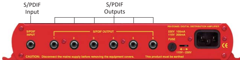
Fig 11-2: RB-DDA6S Rear panel
