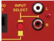
Fig 5-4: RB-DA6RG Input Selector Switch
