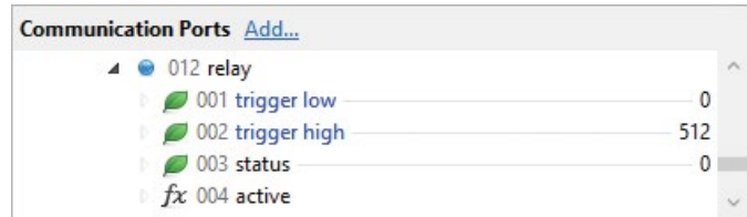
Fig 15-3: Ember+ Relay Node Structure
