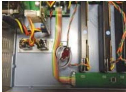
5. Remove the daisy-chained 3 way ribbon cable that connects to channels 5-8 and reposition it so that instead it spans channels 6-9.
