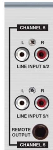
Fig 2-5: Channel 5 Rear Panel Connectors.
