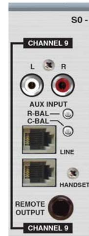
Fig 2-8: Channel 9 Rear Panel Connectors.
