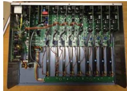
3. Locate jumpers J22, J23 and J24. Reposition the two shorting links to the configuration shown below (use tweezers if necessary):
