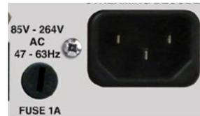
Fig 3-16: PS-PLAY IEC Power Plug & Fuse.
