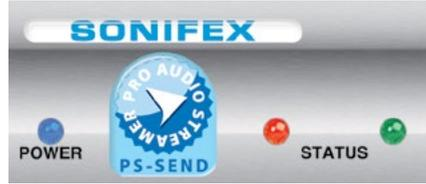
Fig 2-2: PS-SEND Power & Status LEDs
