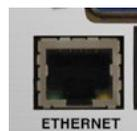
Fig 4-9: PS-AMP ETHERNET Port.
