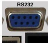
Fig 4-10: PS-AMP RS-232 Serial Port
