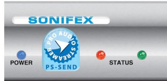
Fig 2-2: PS-SEND Power & Status LEDs
