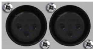
Fig 2-6: PS-SEND XLR Analogue Inputs
