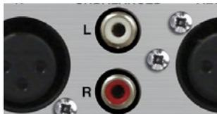
Fig 2-7: PS-SEND RCA Phono Analogue Inputs
