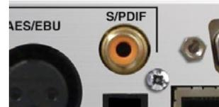
Fig 2-9: PS-SEND S/PDIF Input
