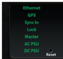
Fig 1-2: Front Panel Indicators
