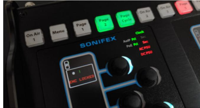
Fig 6-44: Locked encoder
