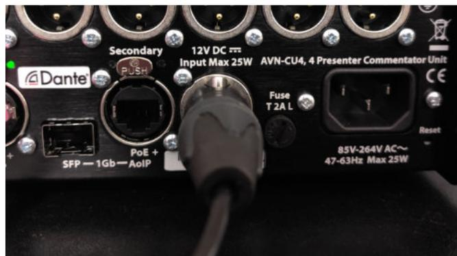
4. If your switch does not support PoE, the DC adaptor can be used instead and has the following pinout:
