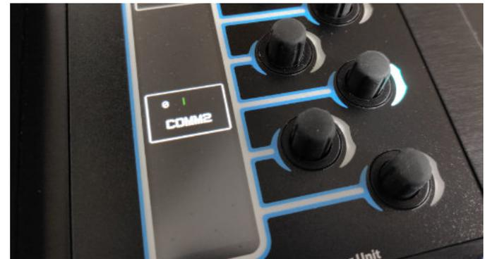
Fig 6-34: Added encoder on the top panel of the device
