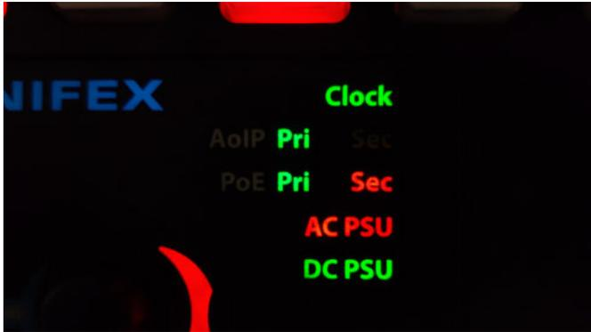
5. When powered using a DC supply, the DC PSU LED will turn green. It is possible to power the unit with PoE and DC at the same time for redundancy.
