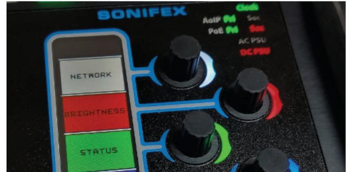
12. Press the 'Menu' button on the front panel of the commentator unit, and select the 'Network' sub-menu by pressing down on the white encoder.
