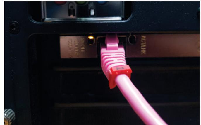
8. Connect an Ethernet cable into the Ethernet port of your PC .
