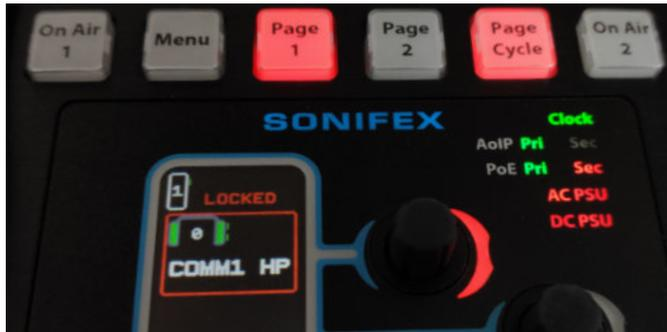
Fig 6-40: Locked user button warning
