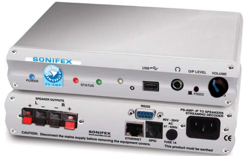
PS-AMP IP to Speakers Streaming Decoder
