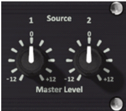
Fig 2-3: AVN-AH8 Master Level Adjust
